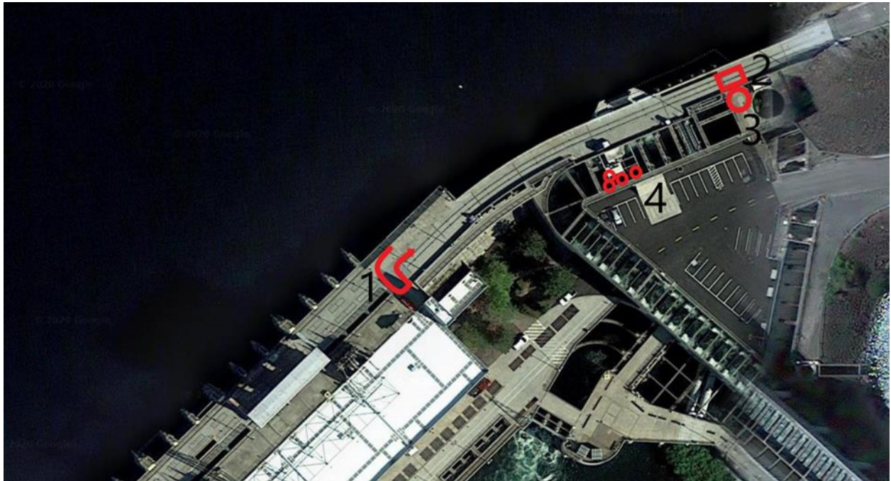
Figure 9. Close-up aerial view of The Dalles Dam East Fish ladder. Small circles (4) denote lamprey tube trap locations above picketed leads. The large red square (2) and circle (3) denote the location of the pulley system used to lift lamprey from the deck of the dam up to the vehicle.
